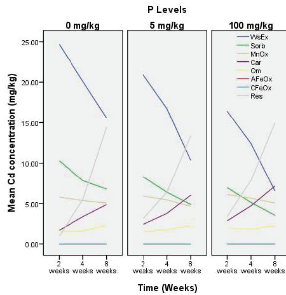
Fig. 4. Effect of phosphorus on cadmium chemical forms in sandy clay loam soil
