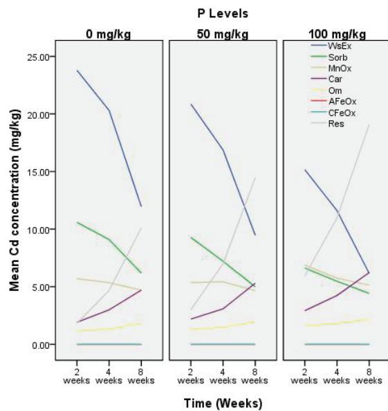
Fig. 3. Effect of phosphorus on cadmium chemical forms in clay soil
