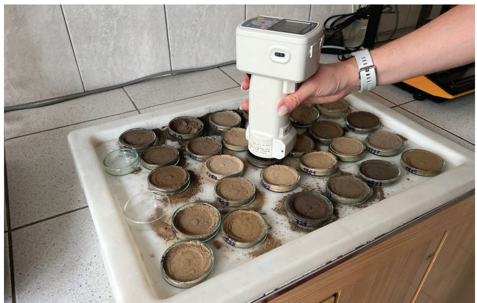
Fig. 1. Laboratory measuring of soil colour in dry soil samples by portable colorimeter.
