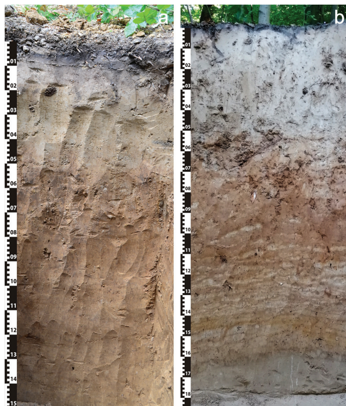
Fig. 1. Gleby płowe typowe (clay-illuvial soils) developed from loess in south-west Poland: (a) profile Henryków – Albic Luvisol (Siltic, Cutanic) and (b) profile Skarszyn forest – Albic Alisol (Siltic, Cutanic)
