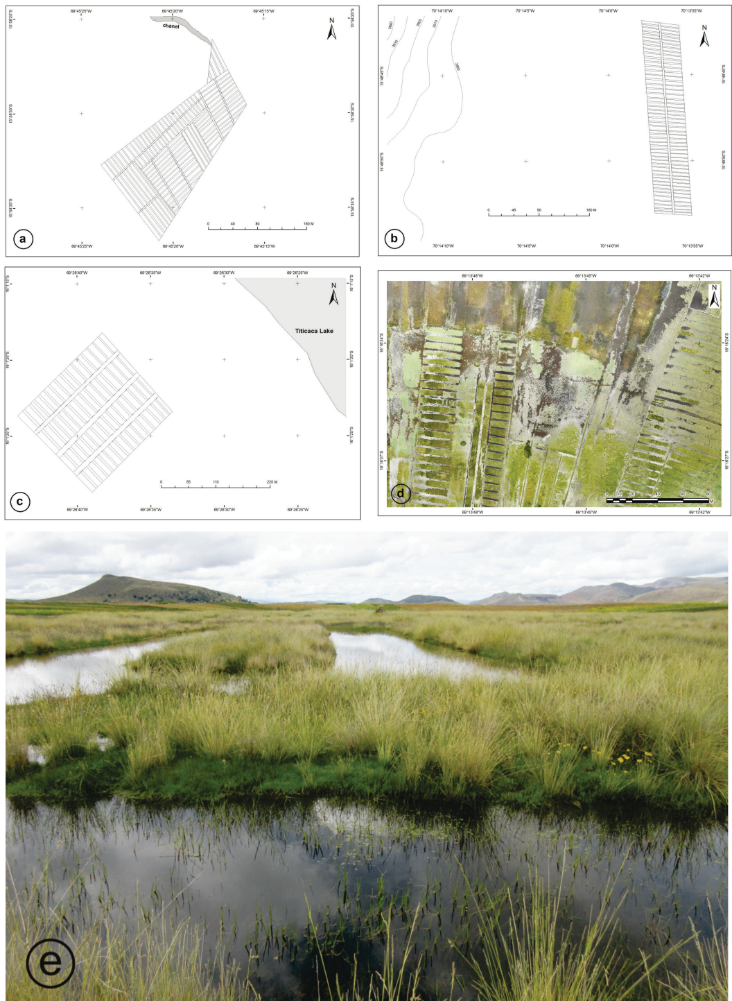
Fig. 2. The Waru Waru system examples. a. Fluvial system, b. Pluvial system, c. Phreatic system, d. Wave image of phreatic system acquired from a drone in the town of Chatuma, district of Pomata.
