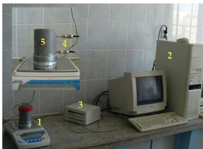
Fig. 2. Laboratory experimental setup for the measurement of soil water retention curve and unsaturated hydraulic conductivity (a, where: 1 – scale, 2 – computer, 3 – pressure head recorder, 4 – two tensiometers, 5 – soil core), and water flux calculation scheme for evaporation method (b, explanation of symbols in the text)
